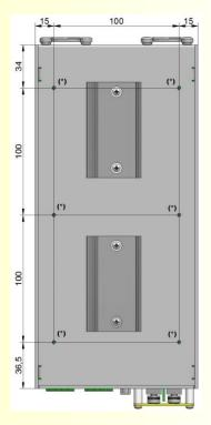
(\*) M3 threaded hole. Maximum screw depth: 3mm
